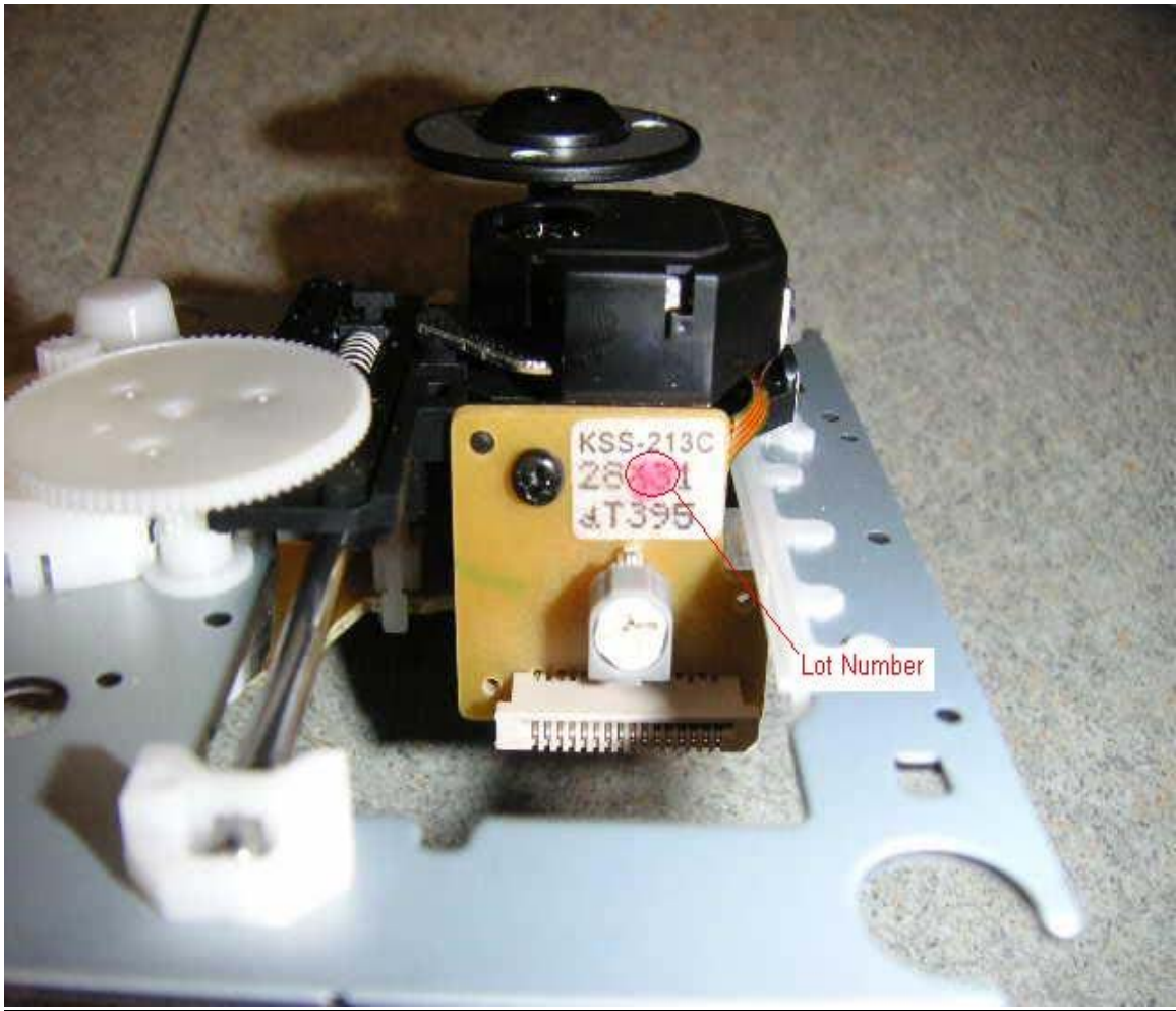
Lot number location on laser pickup.
